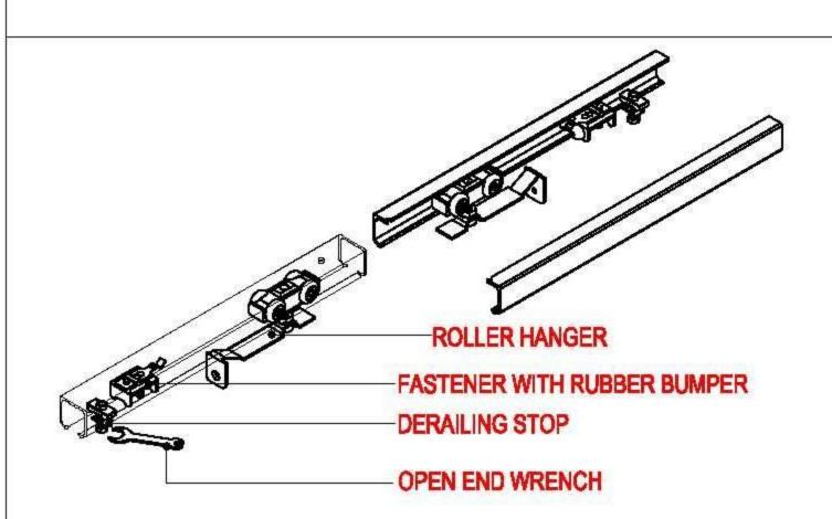
Step 3: Adjust and secure the fastener with slotted screwdriver and the derailing stop with open end wrench to requested location.
