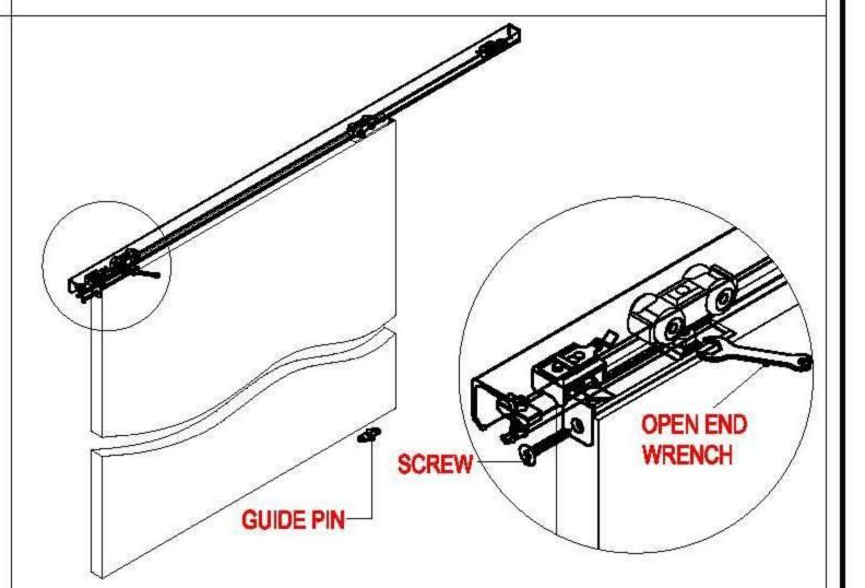
Step 6: Insert plate of the roller hanger into the installation plate and screw it from side of door, keep the door bottom slot align with guide pin. Unlock the nut and adjust the door height by the notch on the screw with open end wrench. Tighten the nuts to lock after the adjustment.
