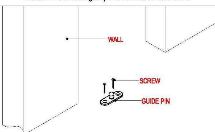
Step 4: Fix the guide pin on the floor to requested location.
