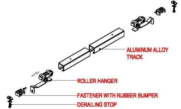
Step 2: Put roller hanger, fastener with rubber bumper, derailing stop into track per the sequence of the DWG. 2 of roller hanger, fastener and derailing stop are needed for each door.
