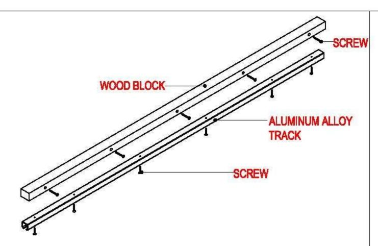
Step 1: Secure wood block to wall with screw first, Screw aluminum alloy track to the bottom of the wood block .
