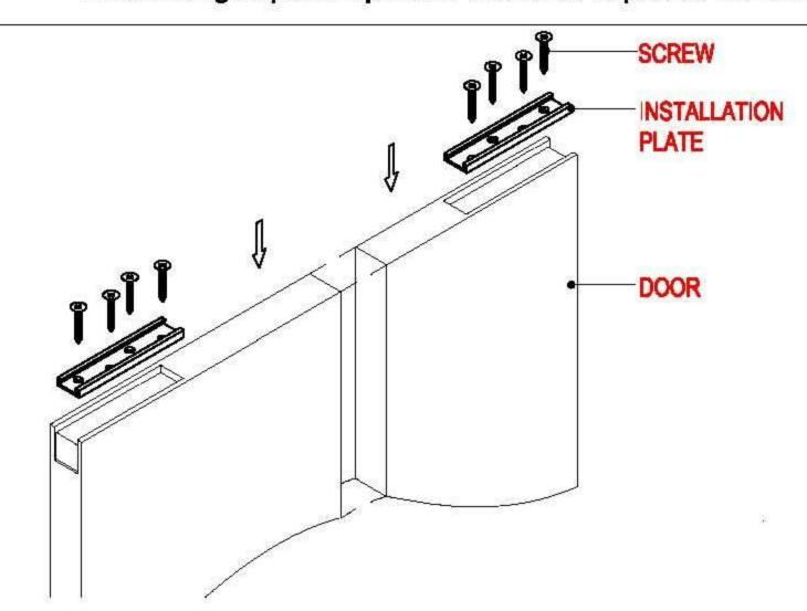
Step 5: Secure the installation plate into the prep-notch on top of door with screw.
